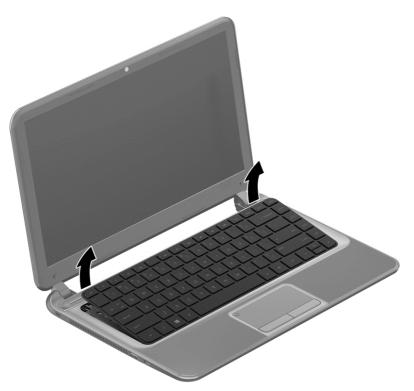
Tilt the keyboard forward (1) onto the palm rest. Release the zero insertion force (ZIF) connector (2) to which the keyboard cable is attached, and then disconnect the keyboard cable (3) from the system board.
